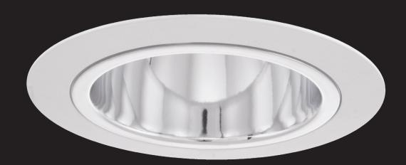
Recessed LED luminaire. Body is made of steel and aluminium and it is available in all RAL colours. Light source - Philips Fortimo LED DLM module. Standard EVG ballast, Touch DALI version on request (please add TD after index number). This LED downlight is also available with 3 hour emergency unit.
