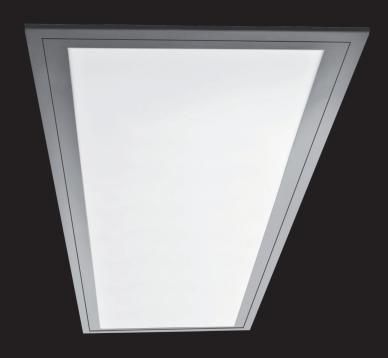
Recessed LED IP44 luminaire with opal diffuser designed for modular ceiling. Light source - Fortimo LED Line Square or Tridonic Stark QLE. Standard EVG ballast, Touch DALI version on request. Body is made of steel and aluminium and is available in all RAL colours. High quality, energy efficient white LED light with CRI 80. Perfect replacement for conventional T5 luminaires. Version for gypsum ceiling on request.
