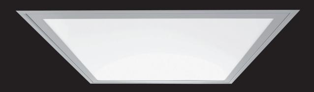
Recessed LED IP44 luminaire with opal diffuser designed for modular ceiling. Light source - Fortimo LED Line Square or Tridonic Stark QLE. Standard EVG ballast, Touch DALI version on request. Body is made of steel and aluminium and is available in all RAL colours. High quality, energy efficient white LED light with CRI 80. Perfect replacement for conventional T5 luminaires. Version for gypsum ceiling on request.
