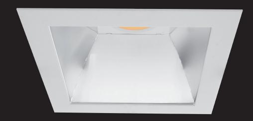
Recessed LED luminaire. Body is made of steel and aluminium and it is available in all RAL colours. Light source - Philips Fortimo LED DLM module. Standard EVG ballast, Touch DALI version on request (please add TD after index number). This LED downlight is also available with 3 hour emergency unit.
