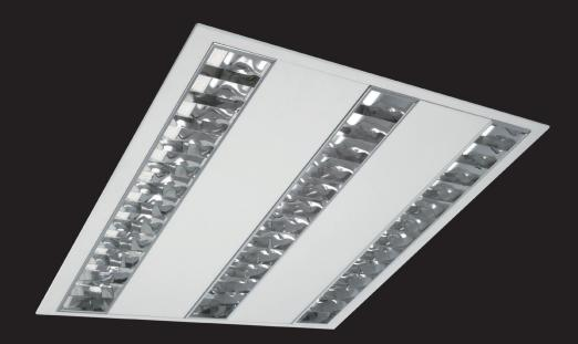
Recessed LED luminaire with parabolic louvers designed for modular or gypsum ceiling. Light source - Fortimo LED Line or PrevaLED Linear. Standard EVG ballast, Touch DALI version on request. Body is made of steel and aluminium and is available in all RAL colours. Version for gypsum ceiling on request.
