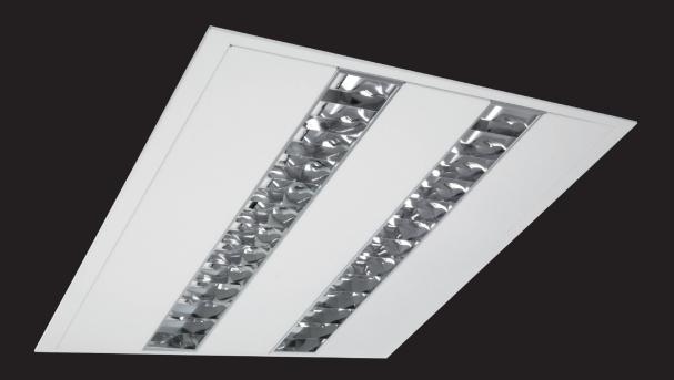
Recessed LED luminaire with parabolic louvers designed for modular or gypsum ceiling. Light source - Fortimo LED Line or PrevaLED Linear. Standard EVG ballast, Touch DALI version on request. Body is made of steel and aluminium and is available in all RAL colours. Version for gypsum ceiling on request.
