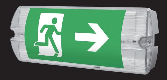
Universal two sided maintained LED emergency lighting fitting. White polycarbonate body, transparent or opal cover. Charging time - 24 hours. Different pictograms on request.
