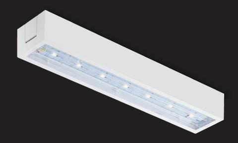
Universal surface mounted maintained LED emergency lighting fitting. White polycarbonate body, transparent cover. Charging time - 24 hours. Different pictograms on request.
