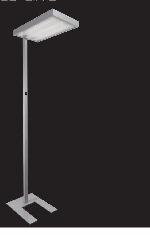
Floor LED luminaire with opal or acrylic diffuser. Light source - Fortimo LED Line, PrevaLED Linear or Tridonic Stark LED module. Standard EVG ballast, DALI version on request. Body is made of steel and aluminium and is available in all RAL colours.
